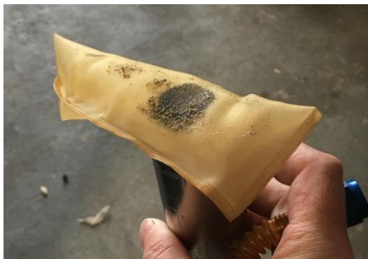
Figure 24 – Example of Dirty In-tank Filter
