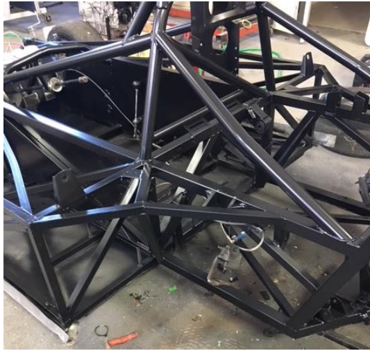
Figure 4 – Frame Stripped and Ready for Modifications
