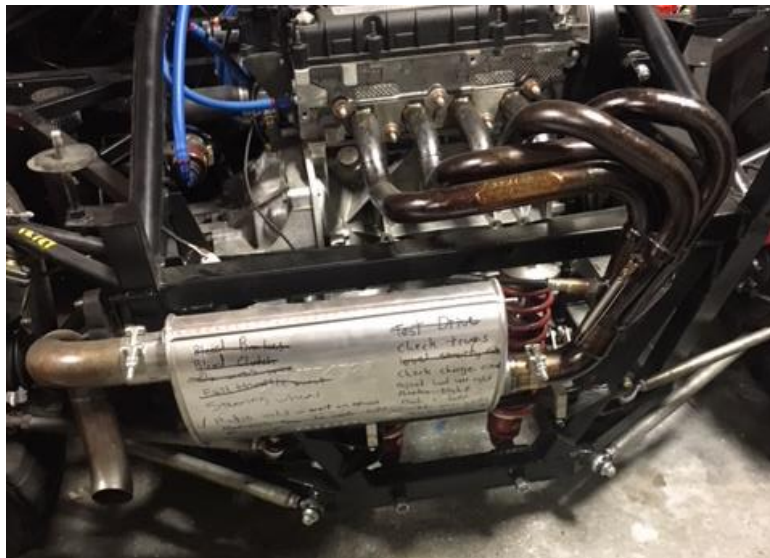
Figure 52 – Muffer and Header Installation
