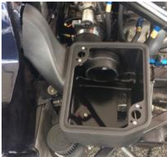
Figure 53 – Air Box Installed
