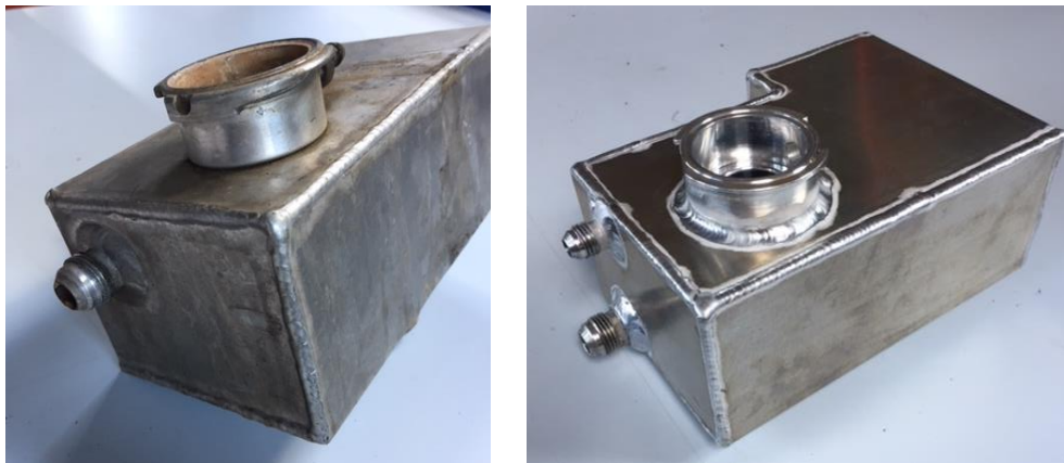
Figure 8 – Un-modified GEN2 & New GEN3 Coolant Tank
