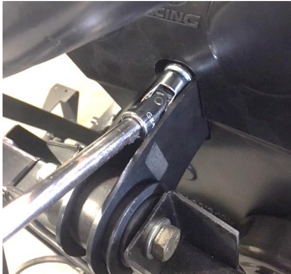
Figure 46 – Tightening the Right Engine Mount Bolts
