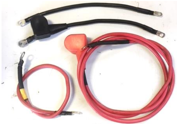
Figure 30 – Modified Ground and Battery Cable
